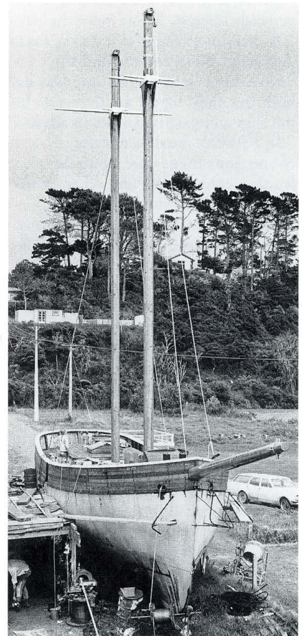
The R. TUCKER THOMPSON building at Mangawhai Heads. Based on a Culler design but with a steel hull
