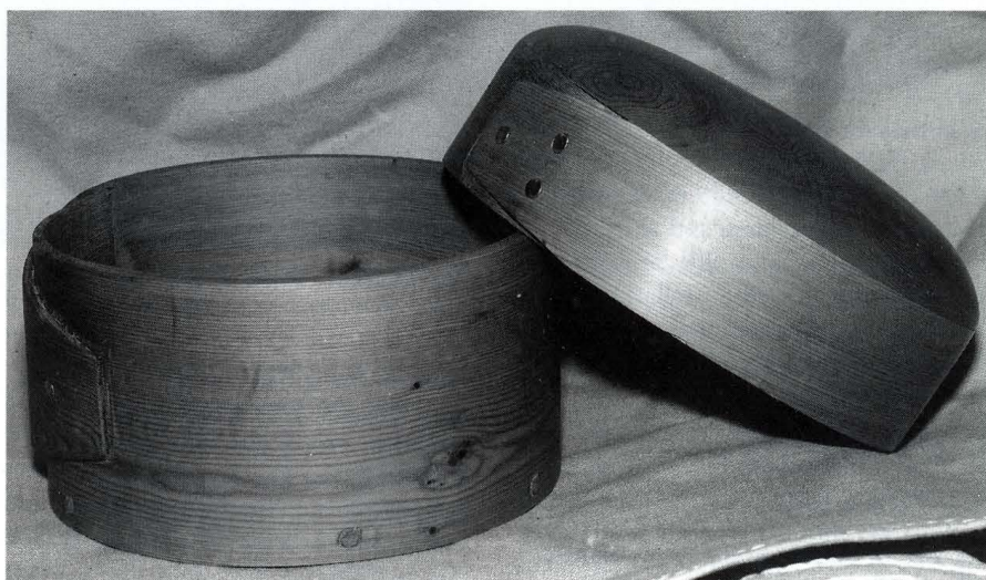
A reproduction of a bent wood ditty box measuring 5.25 inches in diameter by 3.5 inches high, made of Yew wood with brass fastenings.
